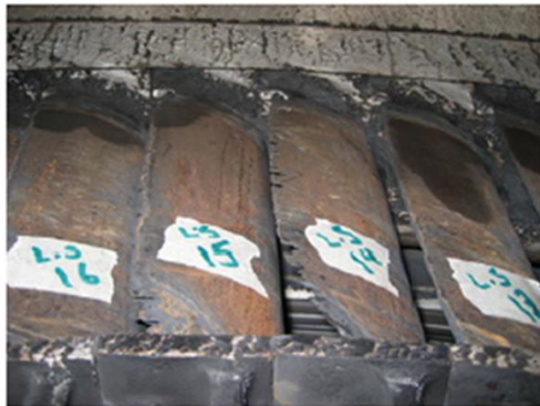
Erosion on the blades as found
