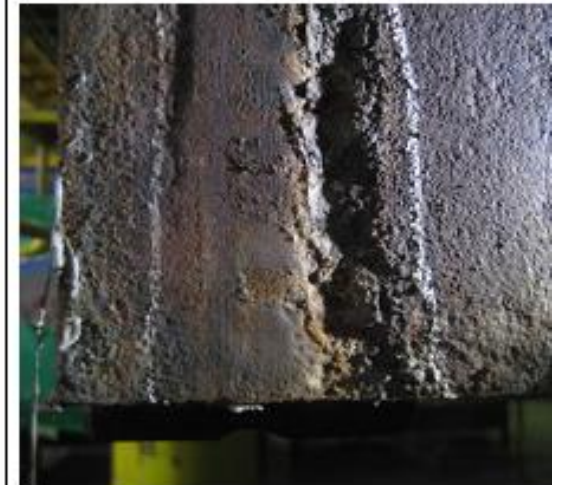
Close up of steam cuts / erosion
