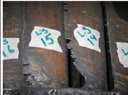
Erosion on the blades as found
